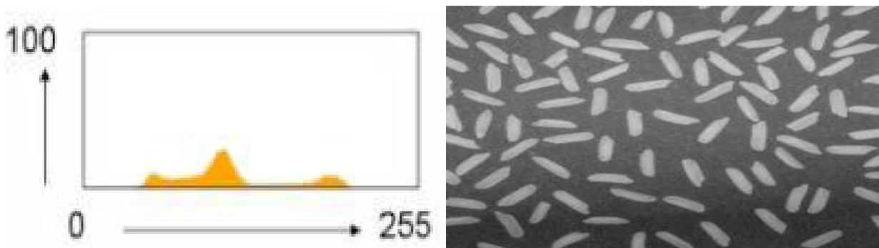
Figure 4: An image with the normalized histogram
