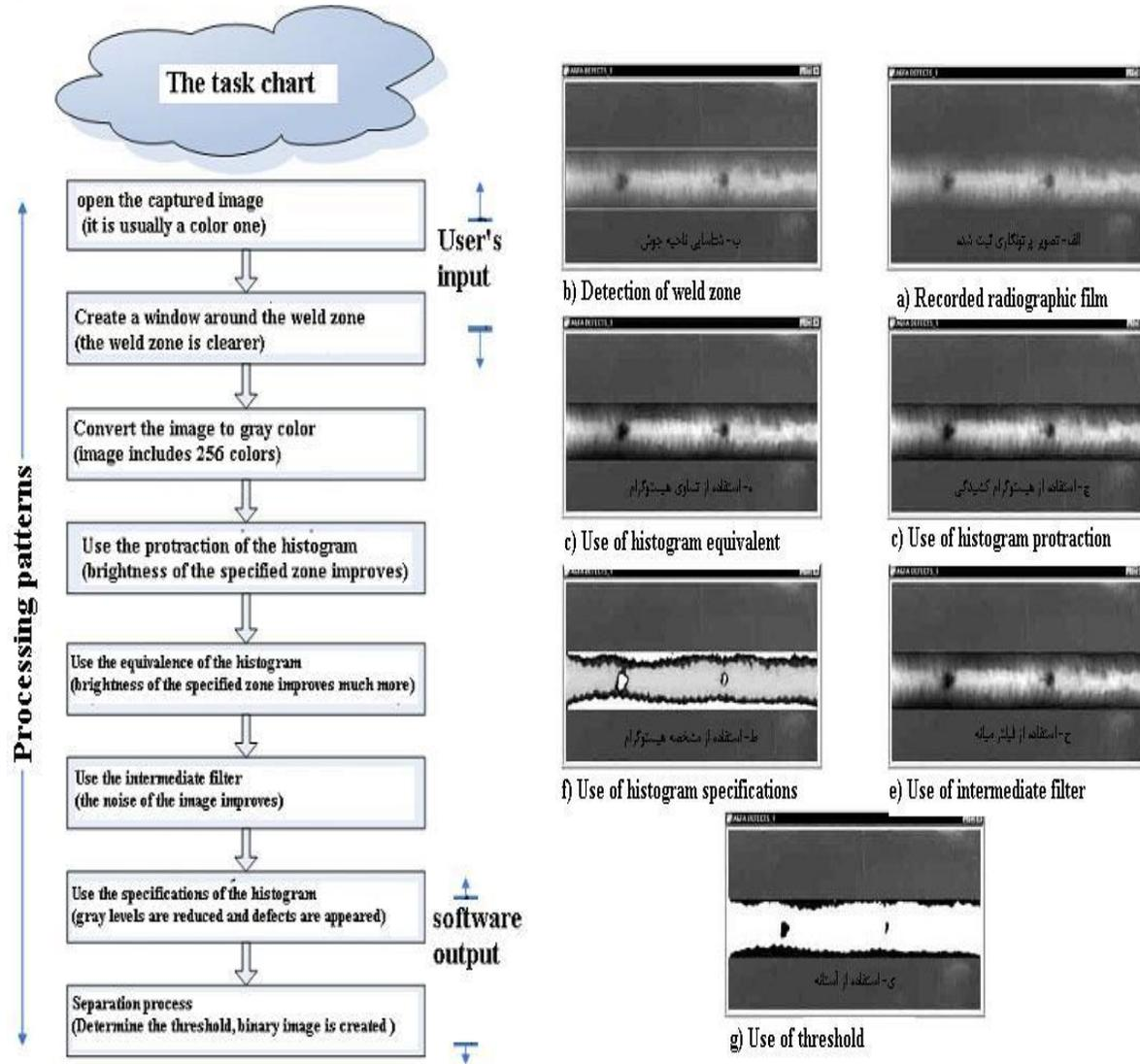
**Figure 6: The main algorithms used to detect weld defects; Fig. (7) The results of system performance on images**
