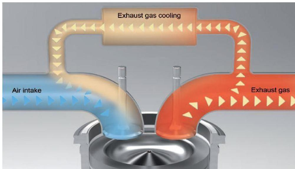
Increased amount of EGR leads to reduced maximum temperature of cycle. The results of this experience show that in addition to reduced NO; UHC and CO pollutants increase in exhaust gas through EGR.
