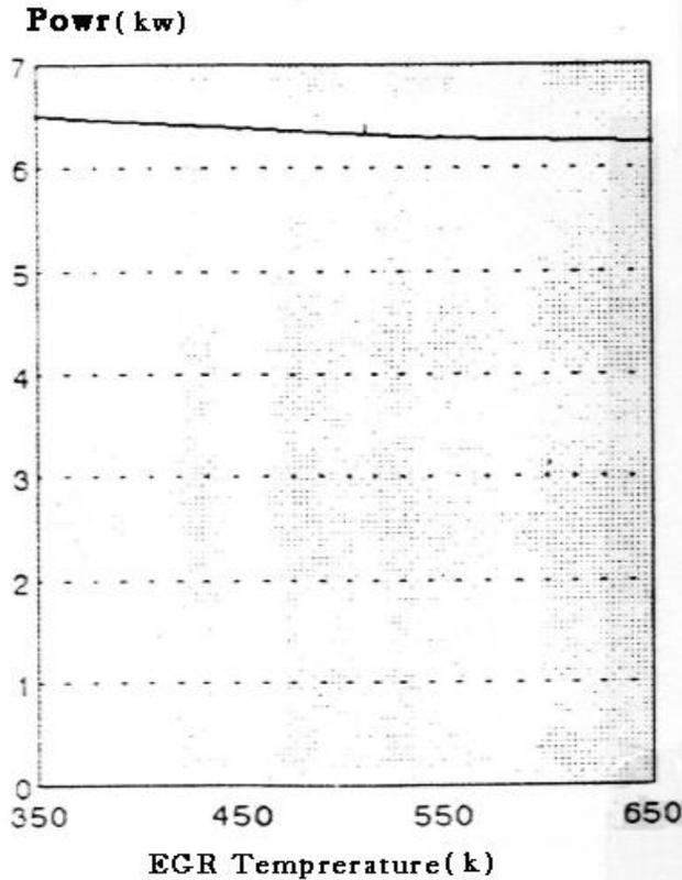
**The effect of EGR temperature on motor power (N=2500 rpm, EGR =10%)**
