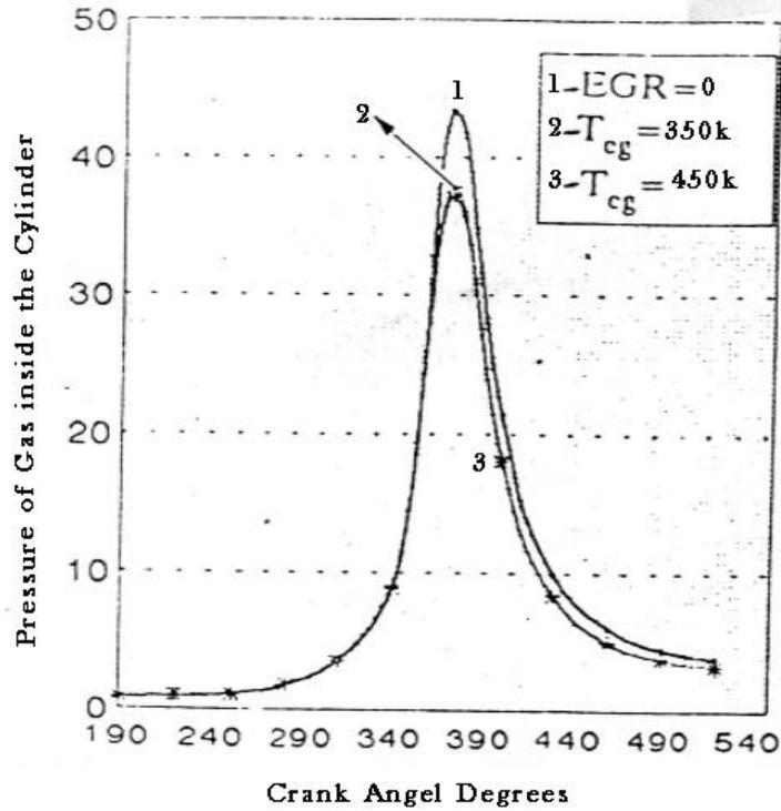
Pressure changes of gases inside cylinder as function of EGR -gas temperature at 2500 rpm
