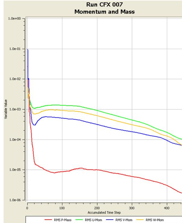
**Figure 5: The curve for changes in residuals based on repetition in periodic model**
