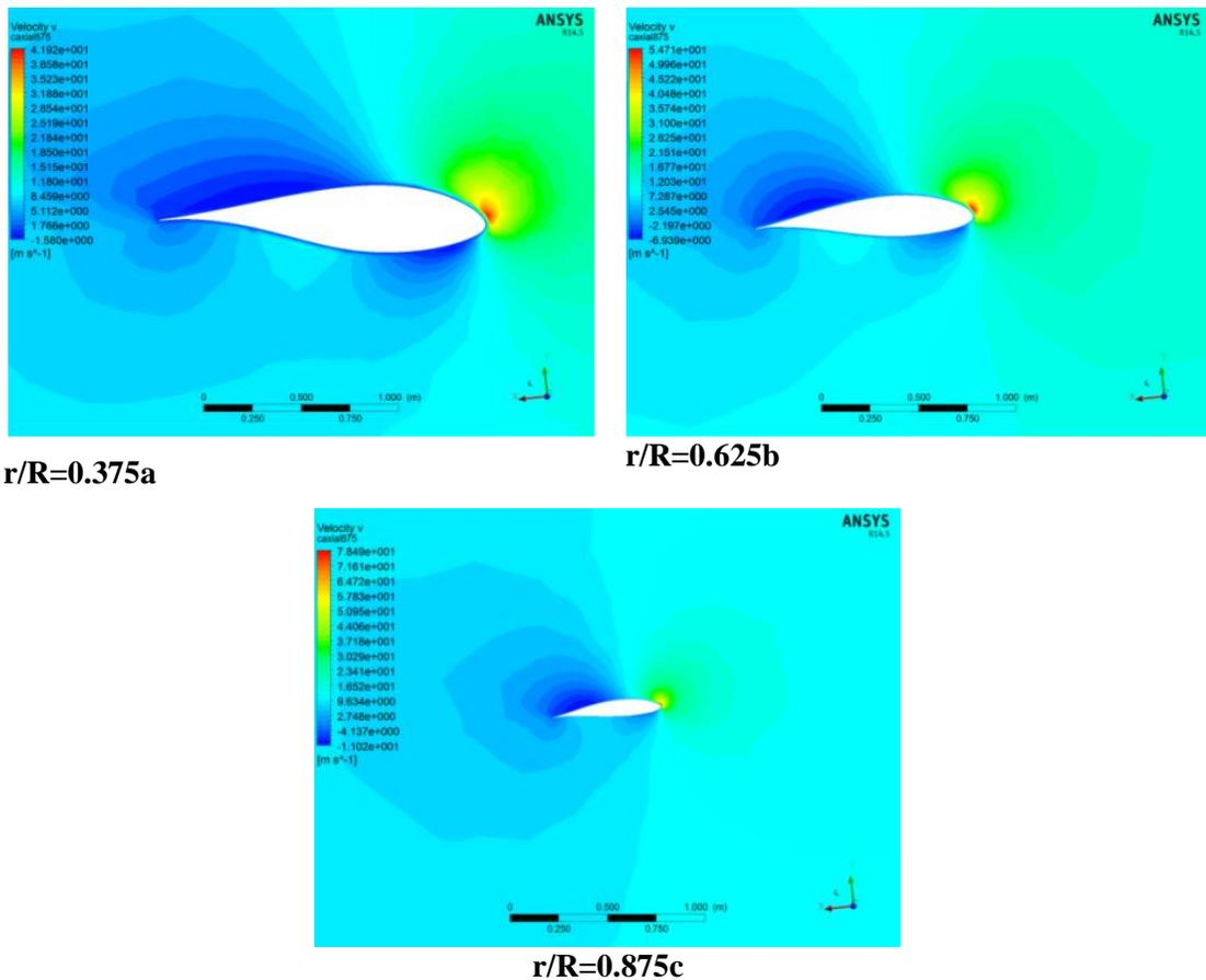
**Figure 8: Axial speed cantor (m/s) at different sections of turbine blade**
