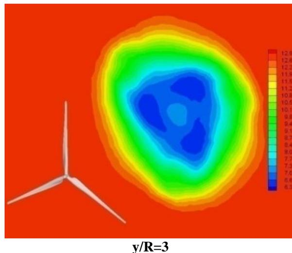
Figure 10: Axial speed contour (m/s) at different distances from turbine
