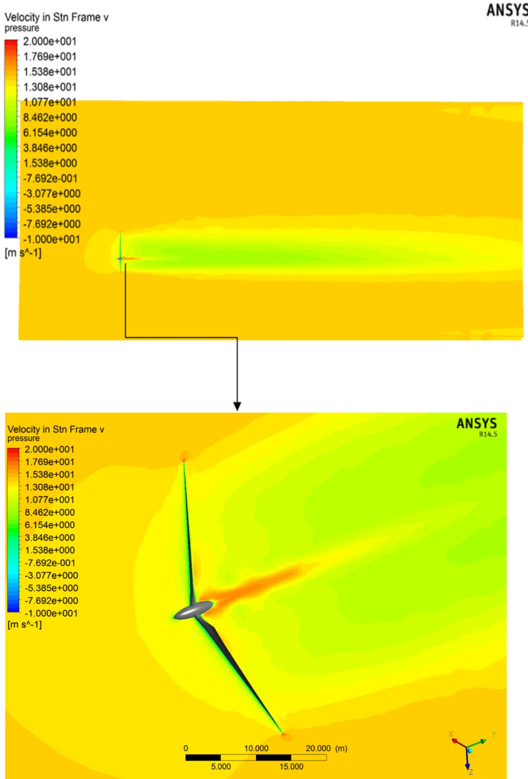
**Figure 9: Axial speed cantor(m/s) at plane which has passed through at the middle of solution(X=0)**
