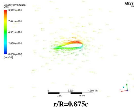
**Figure 7: Relative speed vector at different sections of turbine blade**
