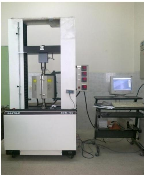
**Figure 6: SANTAM 150KN test apparatus used in the experiments**
