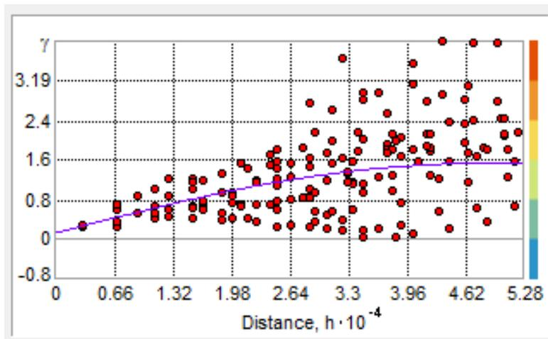
**Figure 2: Fitted Tetraspherical Semivariogram model to 2004 EC dataset**
