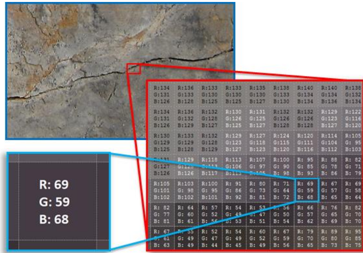
Figure 3: Schematics of joint image pixels disparting to the Red, Green, Blue percentage
