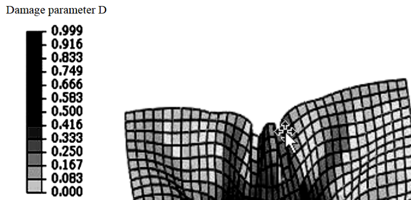
Figure 11: Predictive Result for Sheet with Thickness of 0.8 mm Using Dynamic Criterion
