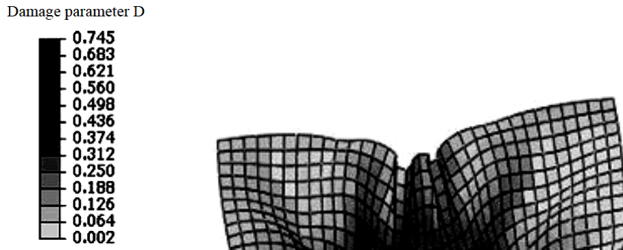
Figure 10: Predictive Result for Sheet with Thickness of 0.8 mm Using Static Criterion
