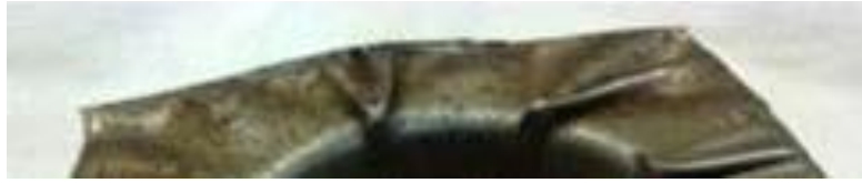
Figure 9: Formed Sheet by Laser Assisted Forming with Thickness of 0.8 mm
