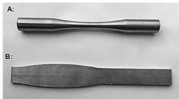
Figure 2: (A) Prepared Steel Specimen for Fatigue Test; (B) Copper Electrode that Used for Forming
